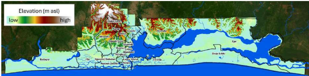
Figure 9: High resolution digital terrain model for Lagos State (LIDAR). Highest elevation above mean sea level at around 70 meters in the Ifako/Ijaye LGA [6]. Figure generated by SwissRe.
