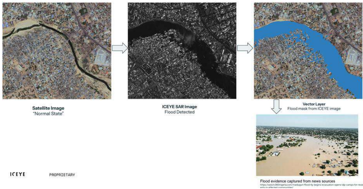
Figure 54: Comparisons of a flood mask from ICEYE SAR imagery with visual confirmations of flooding from the same event in Maiduguri, Nigeria. Figure generated by ICEYE.
