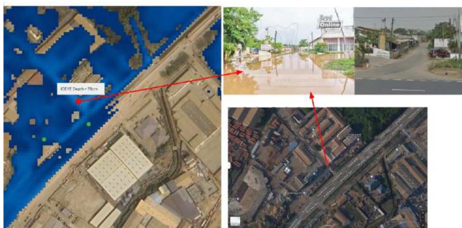
Figure 55: Details of ICEYE's Flood Output of the May 2022 Accra Floods. Blue color scheme shows details of the maximum flood extent in left image. Marked location coordinates are 5.563386, -0.227861, determined at water depth of 76 centimeters. Right top images show the
