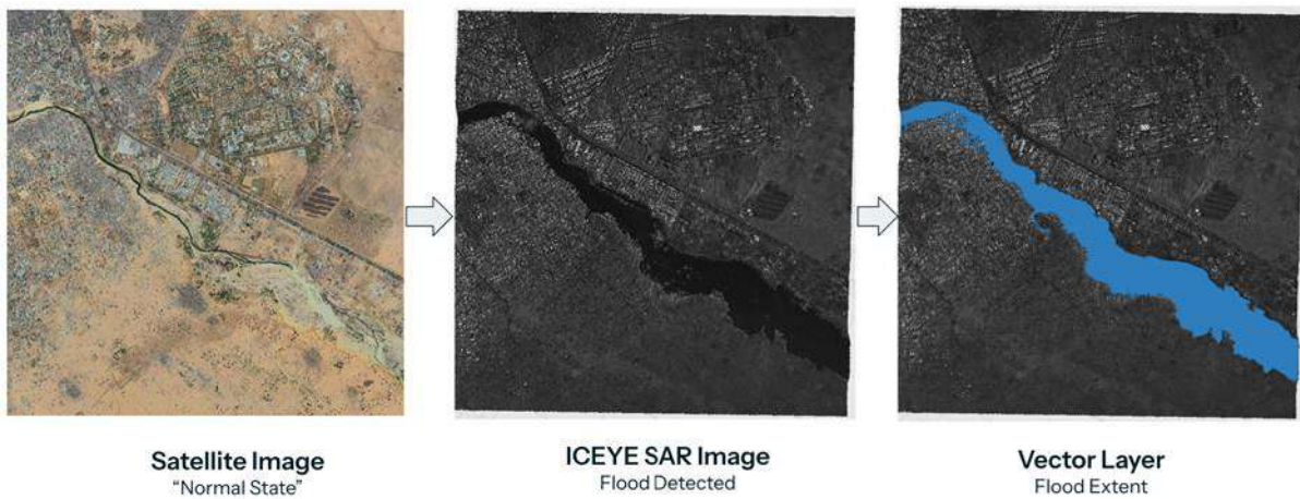
Figure 53: (Top) ICEYE DWELL SAR Image (0.5 m) from Maiduguri, north-east Nigeria, September 2024. (Bottom) Flood mask extracted from ICEYE SAR imagery. Figure generated by ICEYE.
